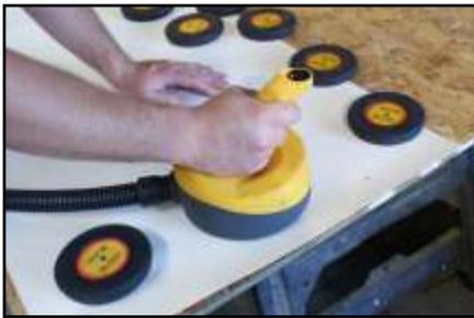
3. Center LED light on handle by moving the handheld in the direction of the lights. Once centered, machine will begin auto-weld. Held still until 'beep' indicates the weld is complete.
